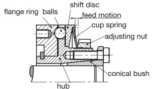
The axial stroke of the shift disc can be used with a proximity or mechanical limit switch for the immediate stop (emergency-OFF) of the drive.
